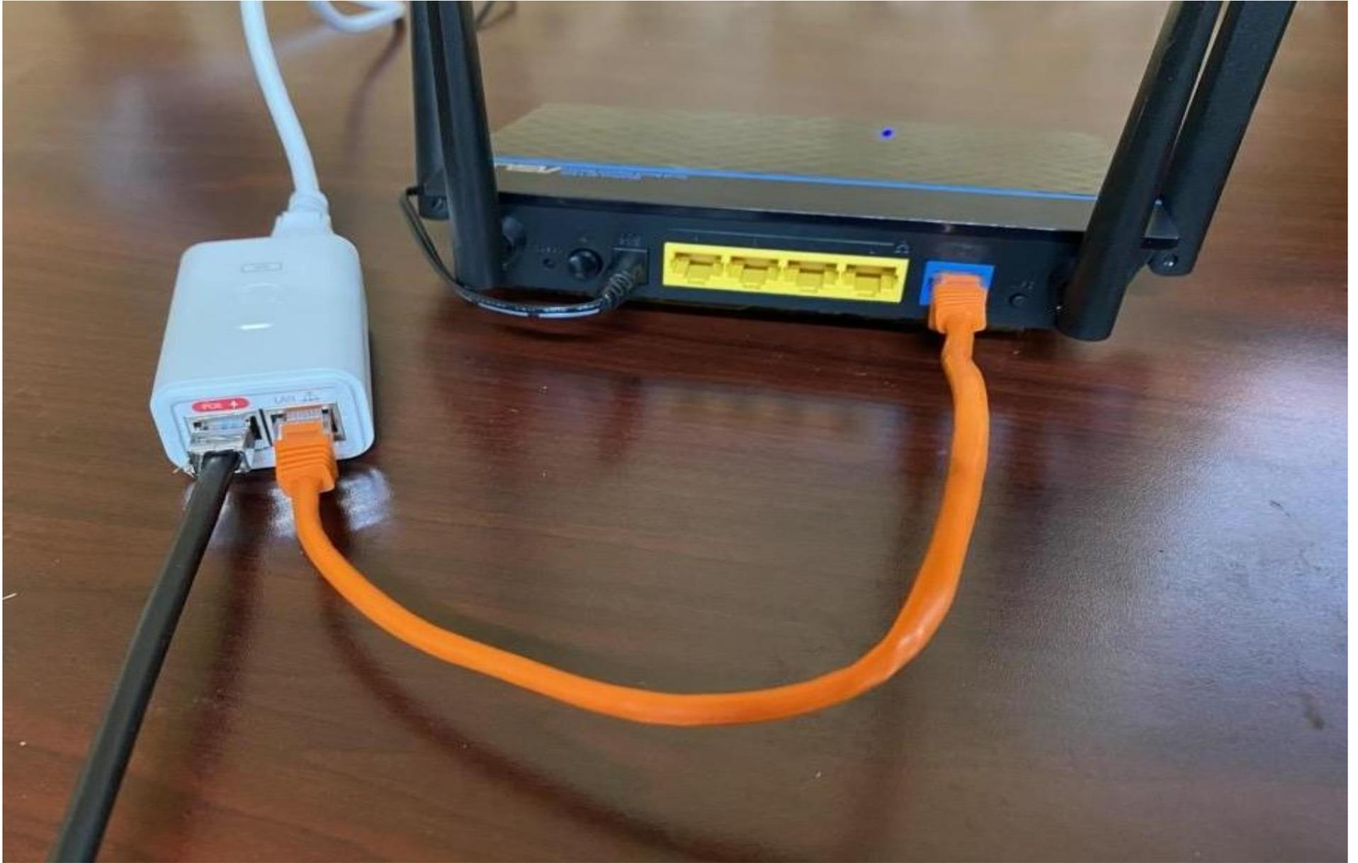
This picture shows how the cable from your power supply's LAN port plugs into the blue port on the back of the TP-Link WIFI router.
